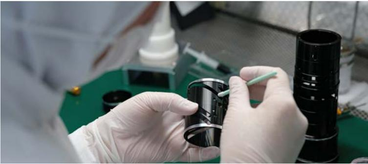
Cam channels in a sub-assembly
