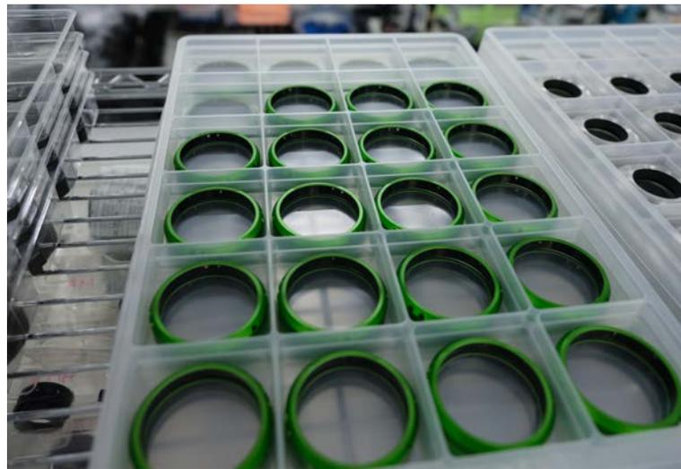
More than 1,000 people work in the vast Fujifilm Taiwa Factory, assembling X-series and GFX cameras, components and other products. A new, dedicated area has been set up for a highly skilled team to build Fujinon MK lenses. The process begins as the various components are gathered, cleaned and checked. Above left: E-mounts. Above right: the distinctive green rear ring.
