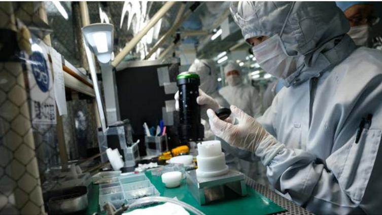
Optical elements are installed into barrel
