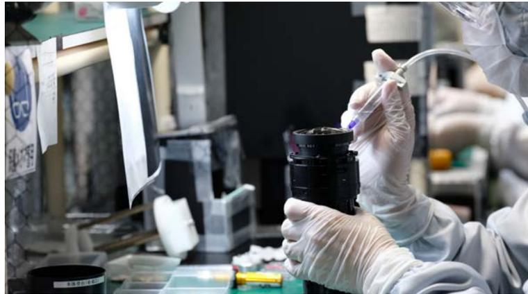
Optical elements are secured in their housings with high-strength cement
