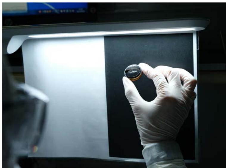
There are 22 optical elements in 17 groups within the MK 18-55. 8 of the elements are ED glass for high optical performance
