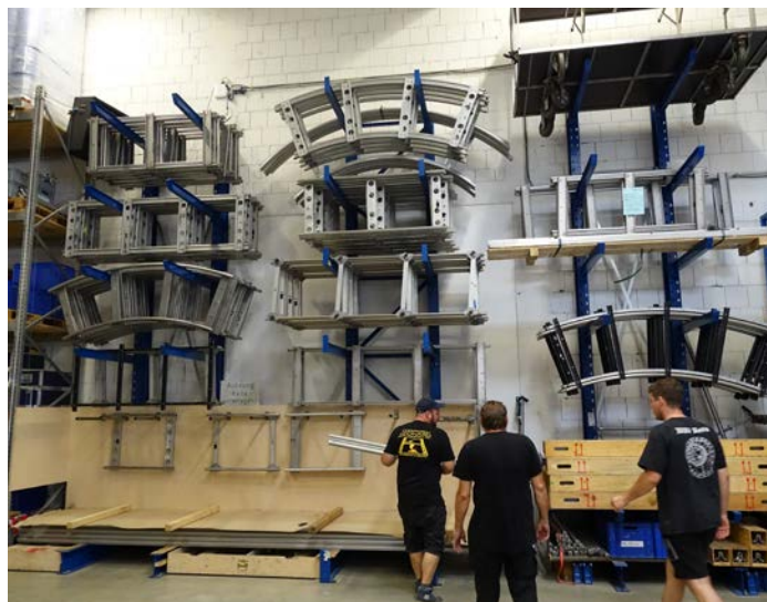
Assembling new dolly track with a unibody triangular frame
