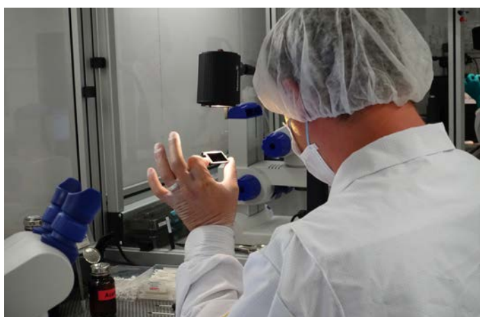
Cleaning individual behind-the-lens ND filters for AMIRA and MINI
