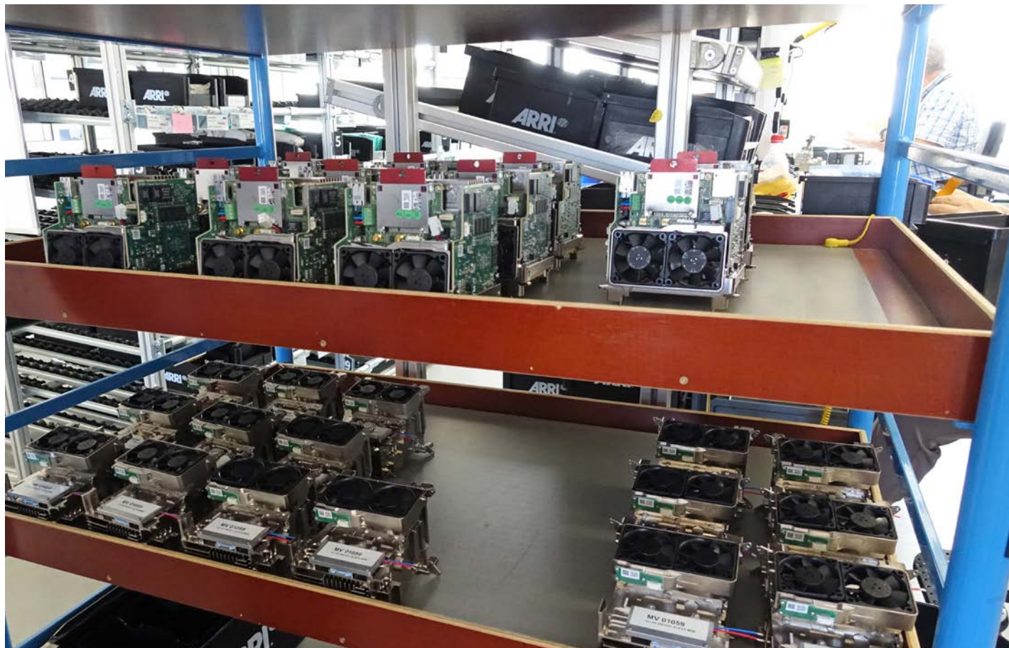
ALEXA Minis in the assembly area (above). ALEXA SXT cameras ready for QC testing (below).
