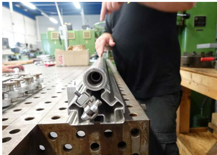
Assembling new dolly track with a unibody triangular frame
