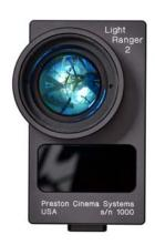
1. Attach the Light Ranger 2 Sensor Unit on top of your camera. Aim it in the same direction as the optical axis of the lens. The LR2 has a 1/4-20 thread on the bottom for easy mounting to a mattebox bar, Schulz Quickfix, or Noga style arm.
