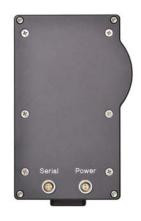
2. Feed the 2-pin POWER connector with 10-30 V DC.
