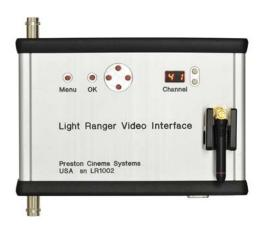
3. The Video Interface Receiver attaches to the back of your viewing monitor. It can connect in-line (BNC HD-SDI or HDMI). The video signal from the camera feeds "Video Input" and "Video Output" connects to the monitor.
